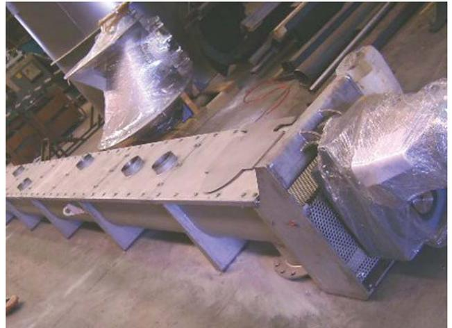
Installation of an Archimedean screw in the plastic industry
