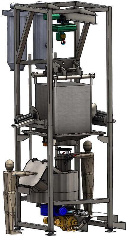
This station allows the big bag and sac emptying independently in a same hopper. This hopper is equipped with a flat-bottom extractor avoiding any phenomenon of bridging, while eliminating the clods of product.
